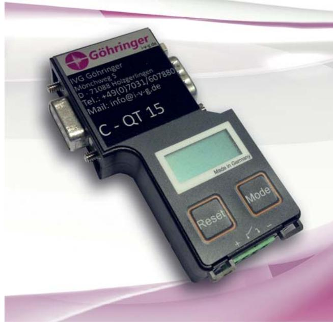
The CAN quick tester C-QT 15 in the form of a D-Sub 9 fieldbus plug provides logical monitoring of CAN bus systems and is integrated into the existing, operating system on a plug-and-play basis. There it automatically detects the baud rate and automatically starts to analyse all bus traffic.
