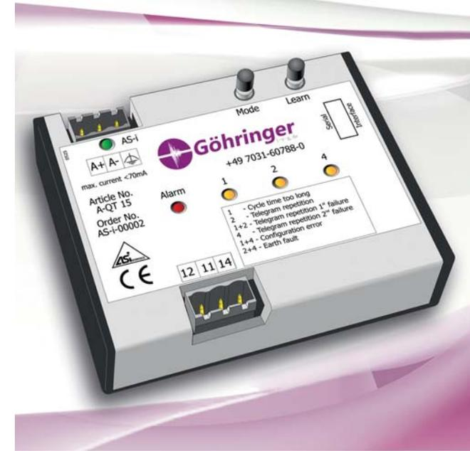
The AS-Interface diagnostic device A-QT 15 is a passive slave on the AS-Interface fieldbus system without its own address. It corresponds to specification V3.0. The diagnostic device monitors data traffic on the network and activates a relay contact for 1 second at a time if it detects a communication error.
