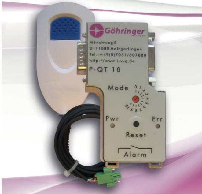
The plug-in diagnosis unit P-QT 10 can be plugged into any Profibus slave, where it will continuously monitor data traffic for typical communication errors. Errors are indicated by the integrated LEDs and reported to higher-level systems by a potential-free alarm contact.
