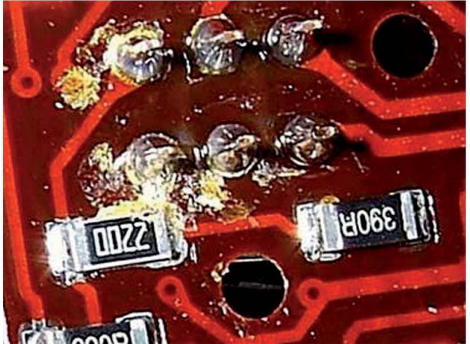
When combined with moisture, flux residues not removed in full become conductive. Image: IVG Göhringer.
