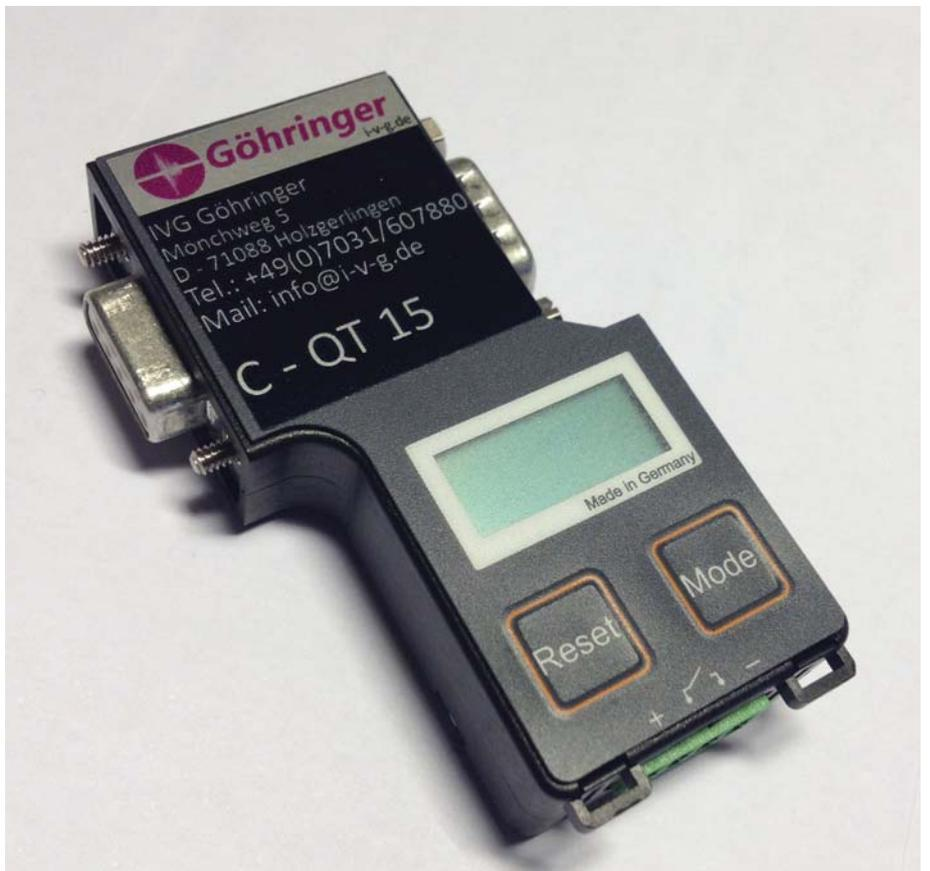
Errors in the CAN communication will be signalled via the integrated status LEDs and an alarm contact. Image: IVG Göhringer.
