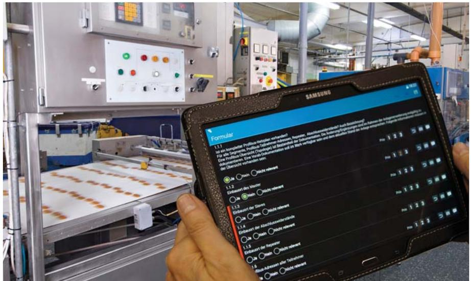
Troubleshooting on the basis of a tablet-supported visual inspection. Image: ©ClarkandCompany/istockphoto.com and IVG Göhringer.
